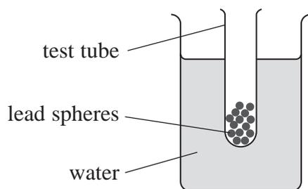
The student gave the test tube a small vertical displacement. The test tube then oscillated vertically.
